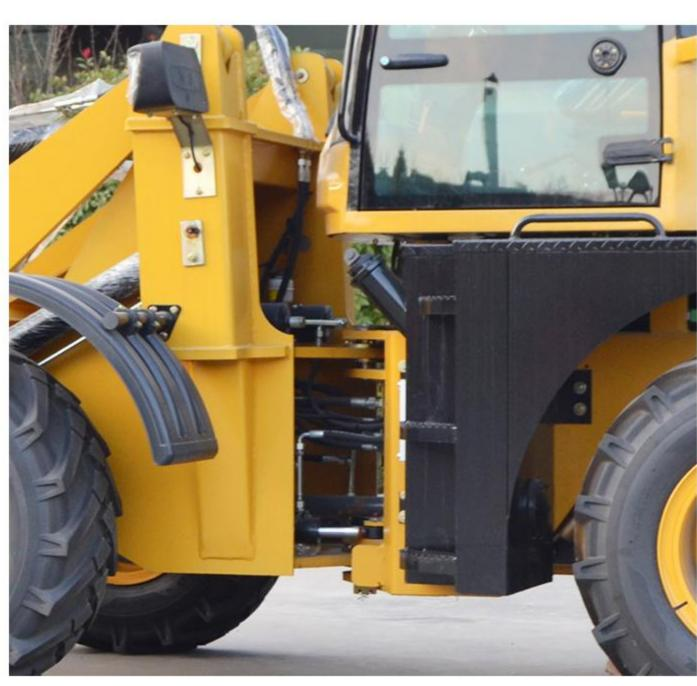
The hydraulic oil tank refueling port and torque converter oil filter are externally located for easy maintenance;
